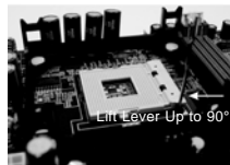
STEP 1: Lift The Socket Lever Up to 90°
