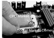
STEP 2/STEP 3: Match The CPU Marked Corner to The Socket Marked Corner
