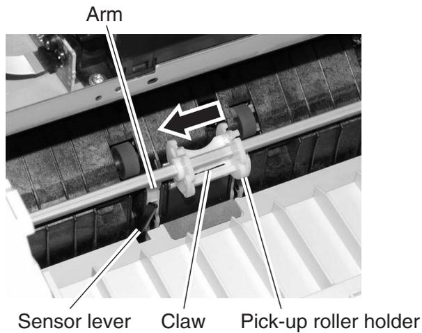
**Figure 3-20 Recording Section 10**
