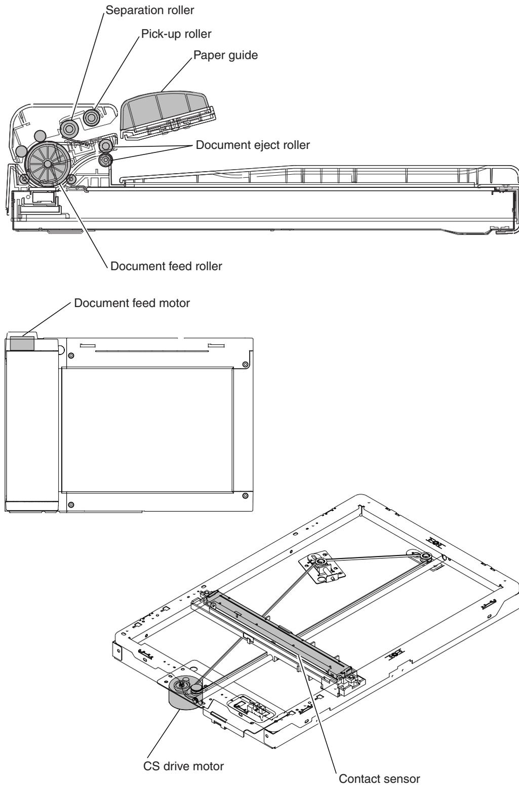
Figure 2-4 Scanner section
