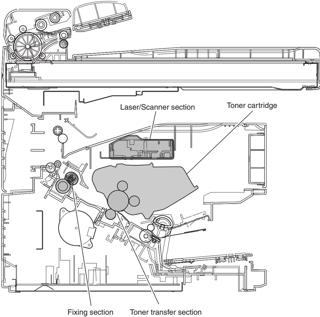
**Figure 2-6 Printer section**
