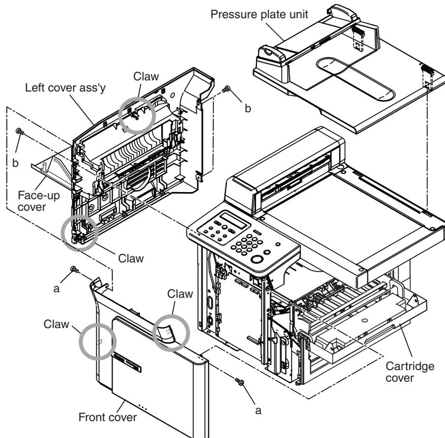
**Figure 3-12 Recording Section 2**
