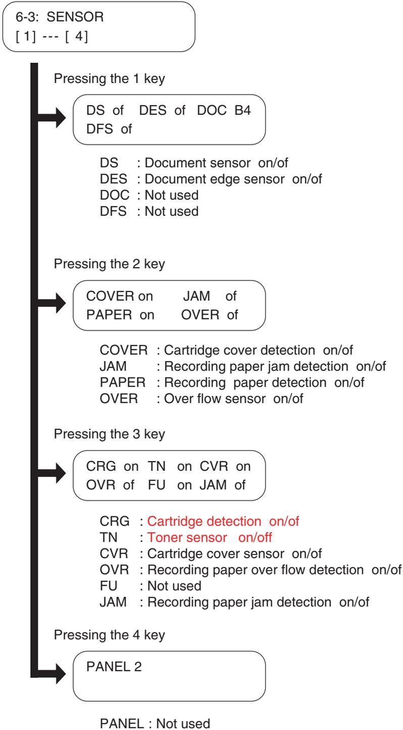
**Figure 4-23 Sensor Tests**
