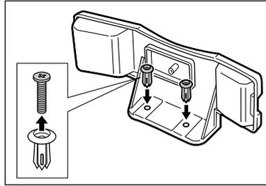
Insert the plugs (with the handset cradle) into the holes on the unit.
