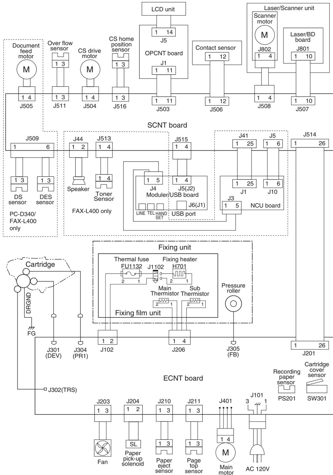
Figure 4-56 Wiring Diagram
