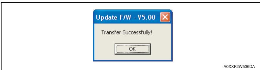
10. Turn OFF and ON the power switch of the machine, and confirm the firmware version. See P.108
