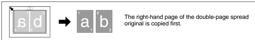
**NARRATION:** A double-page spread original such as a book or magazine is copied onto two separate pages, the image of the original being divided about the mark on the Original Scale. Place the original so that its upper side faces the back side of the machine. Align the center of the original with the mark on the Original Scale. The length of the paper that can be loaded should not exceed 216mm (8-1/2 inches).
