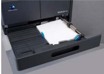
**NARRATION:** This explains the paper feed retry control. To reduce the number of paper feed failures, the paper feed sequence is temporarily halted and a paper feed retry sequence is carried out.
