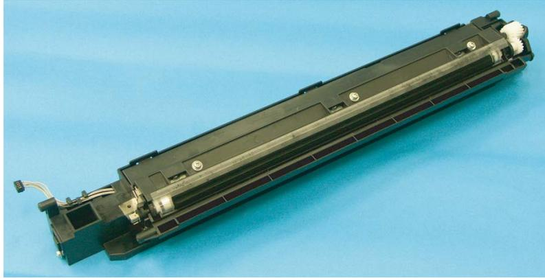
NARRATION: This illustration shows the configuration of the developing section of the imaging unit.
