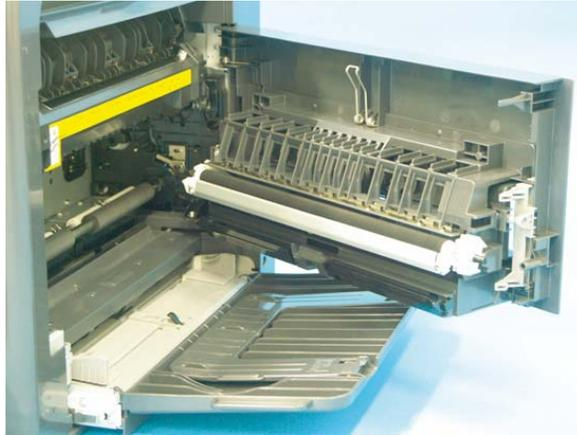
NARRATION: This illustration shows the configuration of the transfer/separation section.
