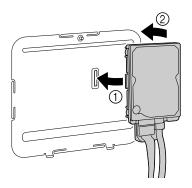
6 Plug the two cables on the Hard Disk Kit HD-P03 into the connector.
