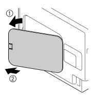
$3 \ \, \text{Using a coin, remove a screw}.$
