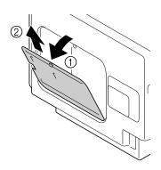
5 Attach Hard Disk Kit HD-P03 to the back of the cover.
