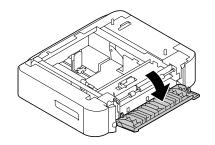
The right side cover of the lower feeder must be opened before the feeder can be installed onto the machine.
