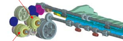
Normal rotation clutch of the Switchback roller
