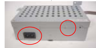
Figure 1-7. Assembling of Shield Plate (Upper)
