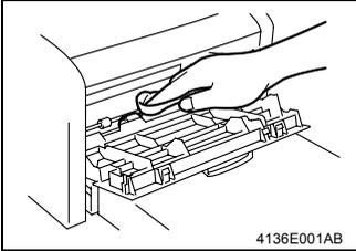
2. Using a soft cloth, wipe the surface of the Paper Take-Up Roll clean of dirt.
