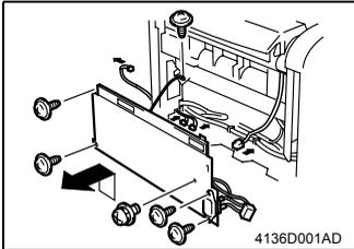
4. Disconnect one connector from the Controller/ Mechanical Control Board.
