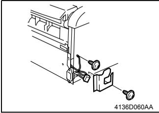
2. Remove two screws and the Power Switch stay.
