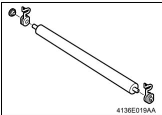
4. Pull out the bushings on the right and left ends, and the gear, from the Image Transfer Roller removed from its holder. Install the bushings and the gear to the new Image Transfer Roller.
