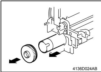
6. Pull out the drive gear from the Fusing Roller.
