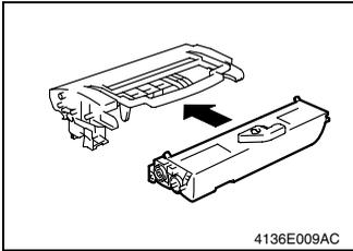
2. Install the new Toner Cartridge to the Drum Cartridge.
