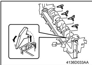
8. Remove the four Fusing Roller Paper Separator Fingers.
