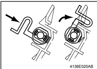
5. Insert the new Image Transfer Roller into the Image Transfer Roller holder and place the levers of the bushings into the original upward positions.
