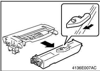
3. Pull the lever of the Toner Cartridge in the direction shown in the illustration and disconnect the Toner Cartridge from the Drum Cartridge.
