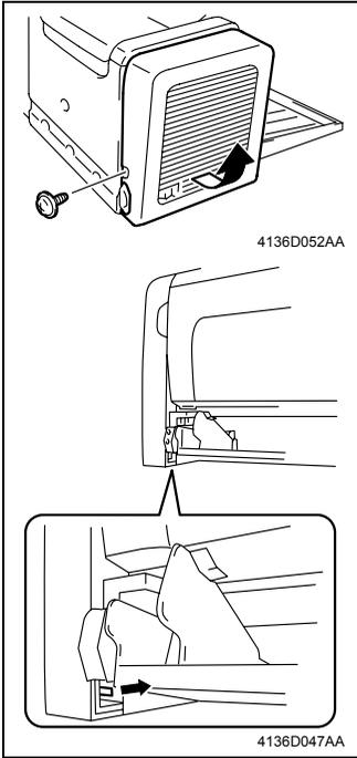
1. Remove one screw, unhook one tab, and remove the Left Cover.
