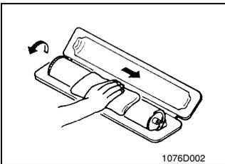
B. Gently wipe the residual toner off the surface of the PC Drum with a dry, Dust-Free Cotton Pad.
