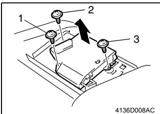
3. Remove three screws and the PH Unit.
