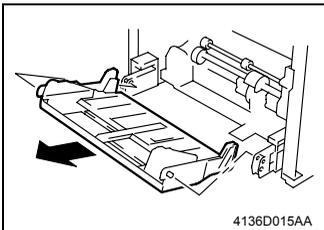
6. Remove the Paper Lifting Plate Assy.
