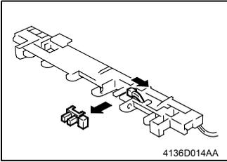
7. Disconnect one connector and remove the Paper Empty Sensor.
