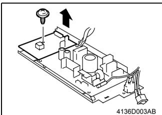
2. Remove one screw and the High Voltage Unit.
