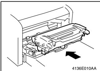
2. Install the Imaging Cartridge in the printer.
