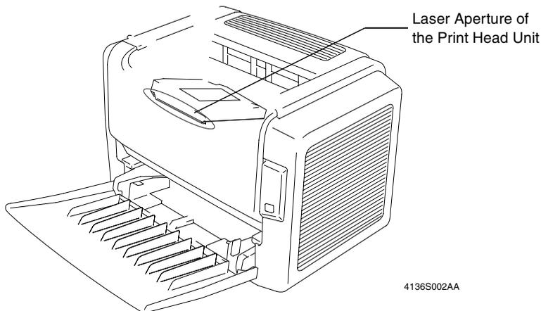
This figure shows the view inside the Front Cover with the Toner Cartridge and the Drum Cartridge removed.
