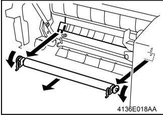
3. Place the levers of the bushings (white) on the right and left ends of the Image Transfer Roller toward this side and remove the Image Transfer Roller from the Image Transfer Roller holder.
