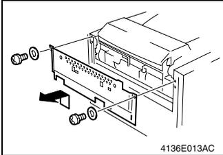
3. Remove two screws and two washers. Then, remove the Fusing Unit protective metal bracket.
