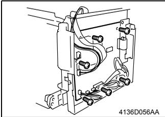
3. Disconnect all connectors and flat cables from the Controller/Mechanical Control Board.
