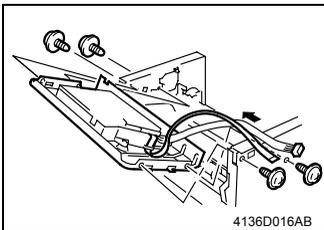
8. Disconnect one connector and one flat cable from the Controller/Mechanical Control Board.
