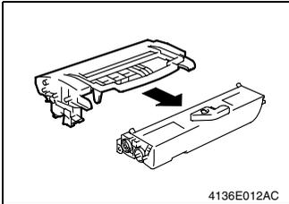
1. Mount the Toner Cartridge to a new Drum Cartridge.
