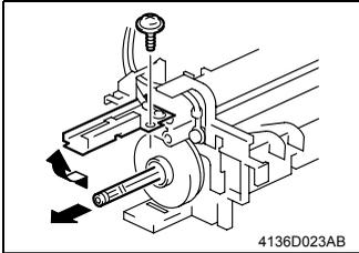
4. Remove one screw and the terminal block.
