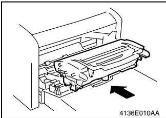
3. Install the Imaging Cartridge in the printer.
