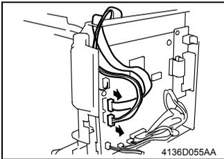
2. Disconnect one connector and one flat cable from the Controller/Mechanical Control Board.
