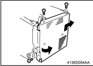
2. Remove three screws and the protective metal bracket.
