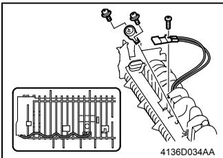
9. Remove one screw and the Thermistor.
