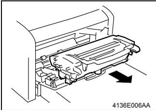
2. Remove the Imaging Cartridge.
