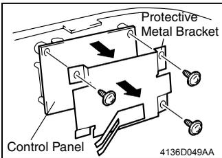
2. Remove three screws, protective metal bracket, and the Control Panel.
