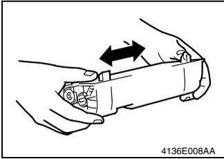
1. Take out a new Toner Cartridge and shake it in the horizontal direction sufficiently so that toner is agitated.
