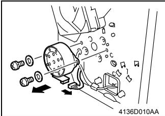
4. Disconnect one connector and remove the Cooling Fan Motor.
