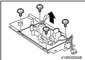
6. Remove four screws and the Power Unit.
