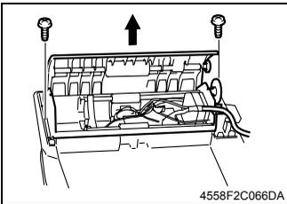
4. Remove two screws and the Drive Unit Assy.
