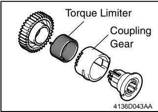
2. Unhook three tabs and take apart the Paper Take-Up Clutch Gear then, remove the Torque Limiter.
