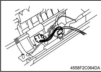
2. Unplug the connector on the AF Control Board and remove the Paper Feeding Sensor Assy.
