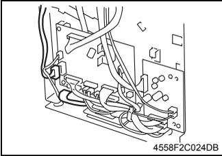
12. Disconnect the flat cable and the connector from the Mechanical Control Board.
