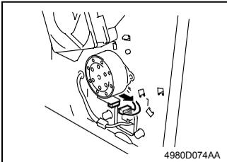
6. Disconnect the connector of the Main Motor.
