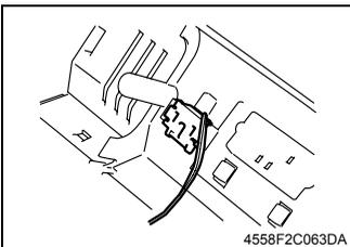
2. Unhook two tabs and remove the Paper Feeding Sensor.
