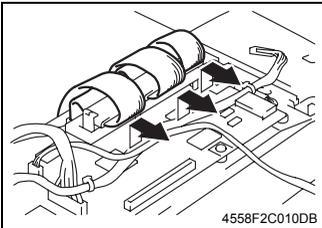
3. Disconnect three flat cables from the Controller/Image Control Board.
