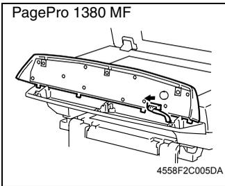
4. Disconnect the connector(s) from the Control Panel.
