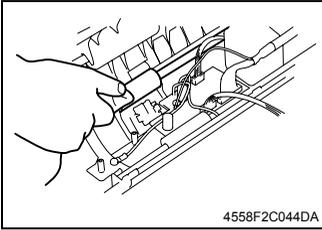
2. Using a soft cloth, wipe clean the surface of the Transport Roller.
