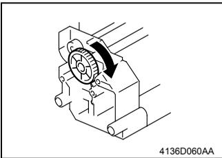
After replacing the Paper Take-Up Clutch Gear (Torque Limiter) on the shaft, rotate the Paper Take-Up Clutch Gear by hand (the Solenoid Flapper needs to be released).
