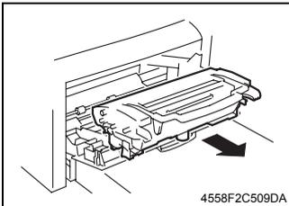
3. Remove the Imaging Cartridge.
