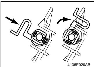
7. Insert the new Image Transfer Roller into the Image Transfer Roller holder and push the levers of the bushings into their original upward positions.
