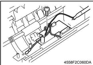
6. Remove the screw, and then remove the AF Control Board.
