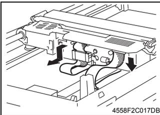
2. Disconnect two Flat Cables from the Scanner Unit.
