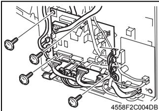
2. Disconnect all connectors and flat cables from the Mechanical Control Board.
