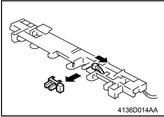
7. Disconnect one connector and remove the Tray 1 Paper Empty Sensor.
