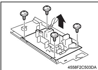
7. Remove four screws and the Power Supply Unit 1.
