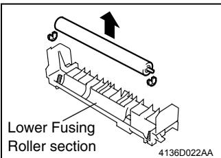
4. Remove two bushings and the Pressure Roller.
