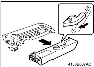
4. Pull the lever of the Toner Cartridge in the direction shown in the illustration and disconnect the Toner Cartridge from the Drum Cartridge.
