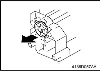
20. Unhook two tabs and remove the Paper Take-Up Clutch Gear.
