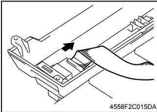
3. Disconnect the flat cables from the Socket Board.
