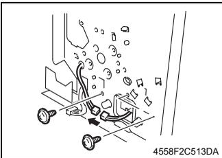
15. Disconnect the connector of the Paper Take-Up Solenoid.
