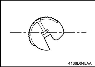
2. When the Roller is leaning in the counter clockwise direction, move the coupling Gear in the B direction.
