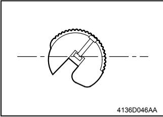
1. When the Roller is leaning in the clockwise direction, move the coupling Gear in the A direction.
