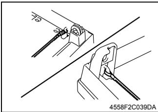
3. Remove the Timing Belt by unhooking it on both sides.
