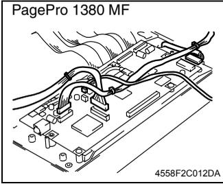
5. Disconnect all connectors from the Controller/Image Control Board.
