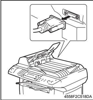
1. Disconnect the ADF connector from the main unit.
