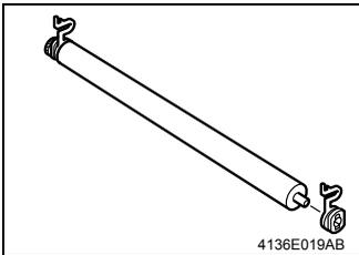
5. Remove the two bushings (one on the right end and one on the left end) and the gear from the Image Transfer Roller.
