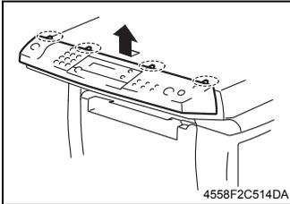
3. Unhook four tabs on the Control Panel.
