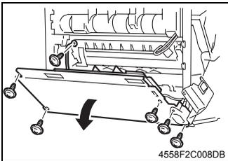
6. Remove six screws, disconnect three connectors, and remove the Power Supply Unit Assy.
