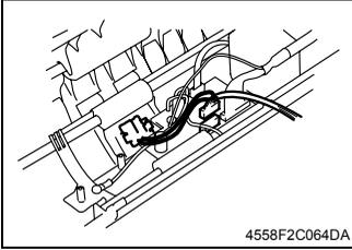
3. Unplug the connector on the AF Control Board and remove the Paper Feeding Sensor Assy.
