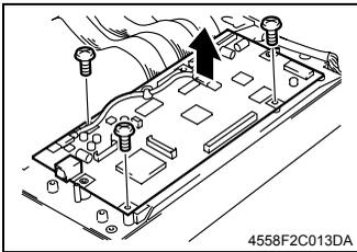
6. Remove three screws and the Controller/Image Control Board.
