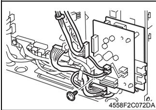
2. Disconnect all connectors and flat cables from the Power Supply Unit 2.
