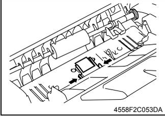
2. Pushing inward the tabs at the front and rear, remove the Separation Pad.
