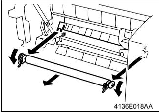
4. Press down the levers of the white bushings (one on the right end and one on the left end of the Image Transfer Roller) and slide the Image Transfer Roller out of the Image Transfer Roller holder.
