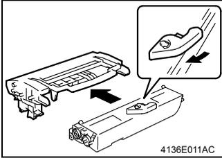
2. Pull the lever of the Toner Cartridge in the direction shown in the illustration and disconnect the Drum Cartridge.
