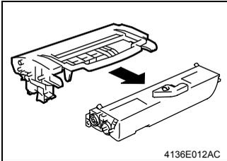
1. Connect the Toner Cartridge to a new Drum Cartridge.
