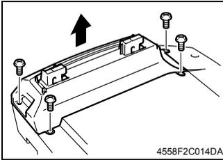
2. Remove four screws and the Socket Board Cover.
