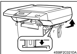
7. Unhook two tabs, and then remove the IR Unit.
