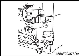
3. Disconnect the connector from the NCU Board.
