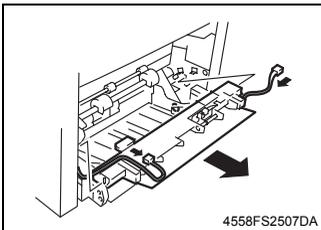
4. Disconnect one connector from the Mechanical Control Board.
