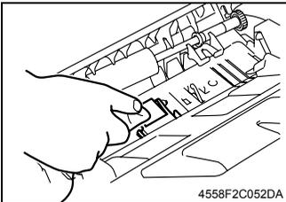
2. Using a soft cloth, wipe clean the surface of the Separator Pad.
