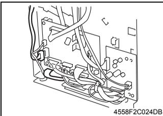
5. Disconnect the flat cable and the connector from the Mechanical Control Board.
