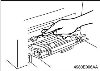
4. Using a soft cloth, wipe the surface of the Paper Take-Up Roller clean of dirt.
