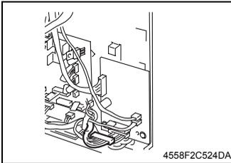
5. Disconnect the connector from the Power Supply Unit 2.
