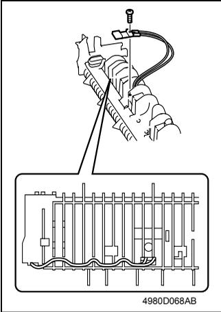
5. Remove one screw and the Thermistor.
