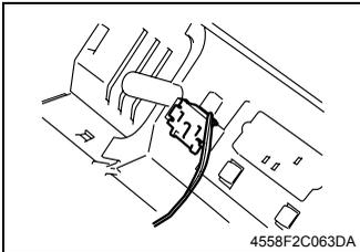
5. Remove the Paper Feeding Sensor and then remove the Auto Document Feeder (ADF) Paper Feed Guide.
