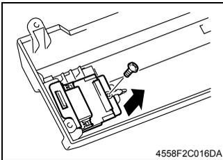
4. Remove the screw and the Socket Board Assy.
