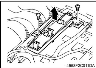
4. Remove two screws and the Flat Cable Guide.
