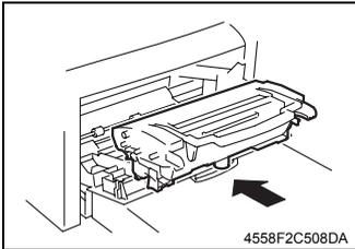
4. Install the Imaging Cartridge in the printer.
