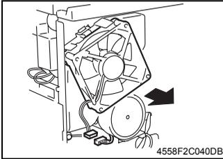
5. Disconnect the connector and remove the Cooling Fan Motor.
