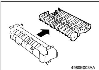
5. Remove the Fusing Unit.
