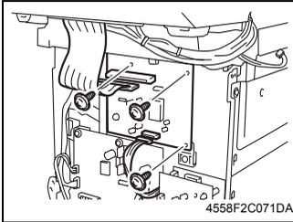
2. Disconnect two connectors from the Interface Board.
