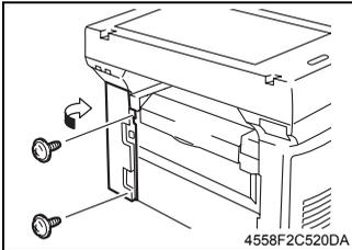
1. Remove two screws that secure the Right Cover at the back and unhook it on the back.
