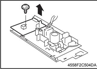
2. Remove the screw and the High Voltage Unit.
