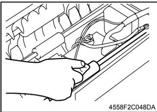
2. Using a soft cloth, wipe clean the surface of the Exit Roller.
