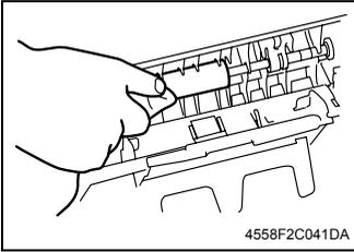
2. Using a soft cloth, wipe clean the surface of the Take-up Roller.
