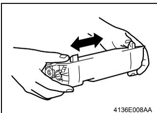
1. Take out a new Toner Cartridge and shake it in the horizontal direction sufficiently to agitate the toner.
