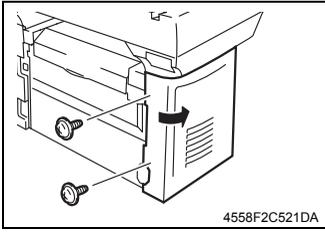
1. Remove two screws that secure the Left Cover at the back and unhook it on the back.
