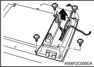
2. Remove four screws and the Controller/Image Control Board Cover.
