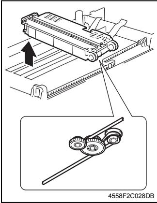
4. Remove the Belt from the Scanner Unit.
