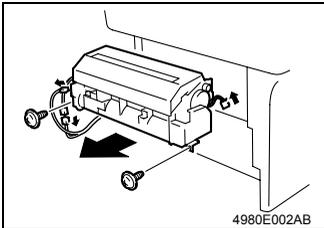
4. Remove two screws, unplug three connectors, and remove the Fusing Unit.
