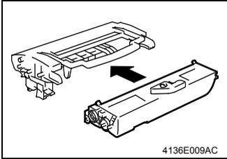
3. Connect the new Toner Cartridge to the Drum Cartridge.
