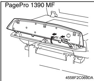
**(6) Removing the Interface Board (PWB-FAX1) <PagePro 1390 MF only>**
