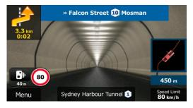
The top-down overview of the tunnel helps you orientate yourself. The remaining distance in the tunnel is also displayed.
