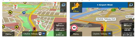
The data fields are different when you are navigating an active route and when you have no specified destination (the orange line is not displayed).
