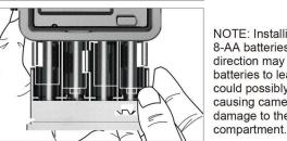
NOTE: Installing any of the 8-AA batteries in the wrong direction may cause the batteries to leak acid and could possibly explode, causing camera failure and damage to the battery
